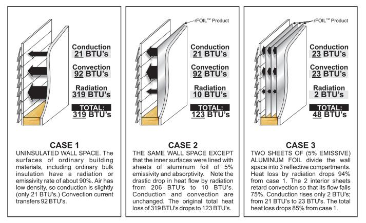
NOTE: 65% (206) BTU's going through this wall space is radiation. Aluminum has 3% to 5% emissivity and absorptivity.
