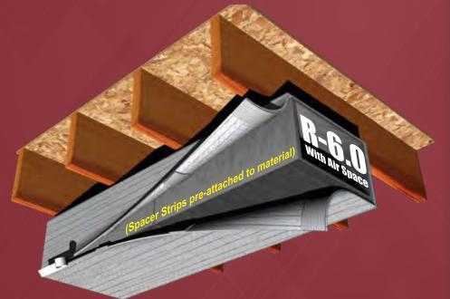
**rFOIL**® BIG-6 Reflective Duct Insulation is a 5/16" layer of polyethylene bubble, bonded to and sandwiched between two highly reflective metalized film surfaces. Four strips of spacers are pre-attached and run along the full length of the roll. These spacers provide the necessary airspace to achieve an R-6.0 insulating value.
