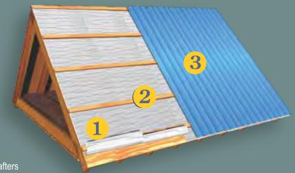
To receive the full benefit from foil insulation, an air space must be created between the panels and the reflective surface of the insulation. Insulation should be stapled down and covered over with 1x4 or 2x4 purlins ahead of the application of the exterior covering.
